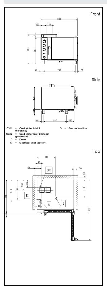
Electric Supply voltage: 260813 (EFCG61CSAS) 220-230 V/1 ph/50 Hz 0.35 kW Electrical power max.: Capacity: Trays type: 6 - 1/1 Gastronorm **Key Information:** External dimensions, Width: 860 mm External dimensions, Depth: 767 mm External dimensions, Height: 701 mm Net weight: 92.1 kg Functional level: Basic Cooking cycles - airconvection: 300 °C Heating-up time (hot air 215°C / 350s. cycle):
